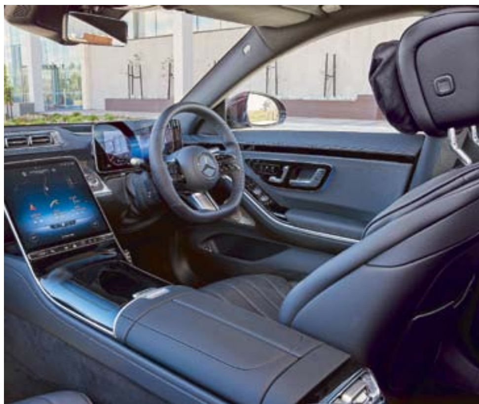
A large central display features OLED (Organic Light Emitting Diode) technology. Positioned in portrait format, it is within easy touch and vision between the driver and front passenger.
