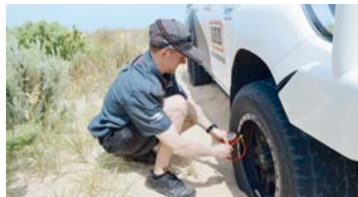
GETTING TYRE PRESSURES RIGHT: Darren said letting tyres down to 18-20psi is always a good idea.
