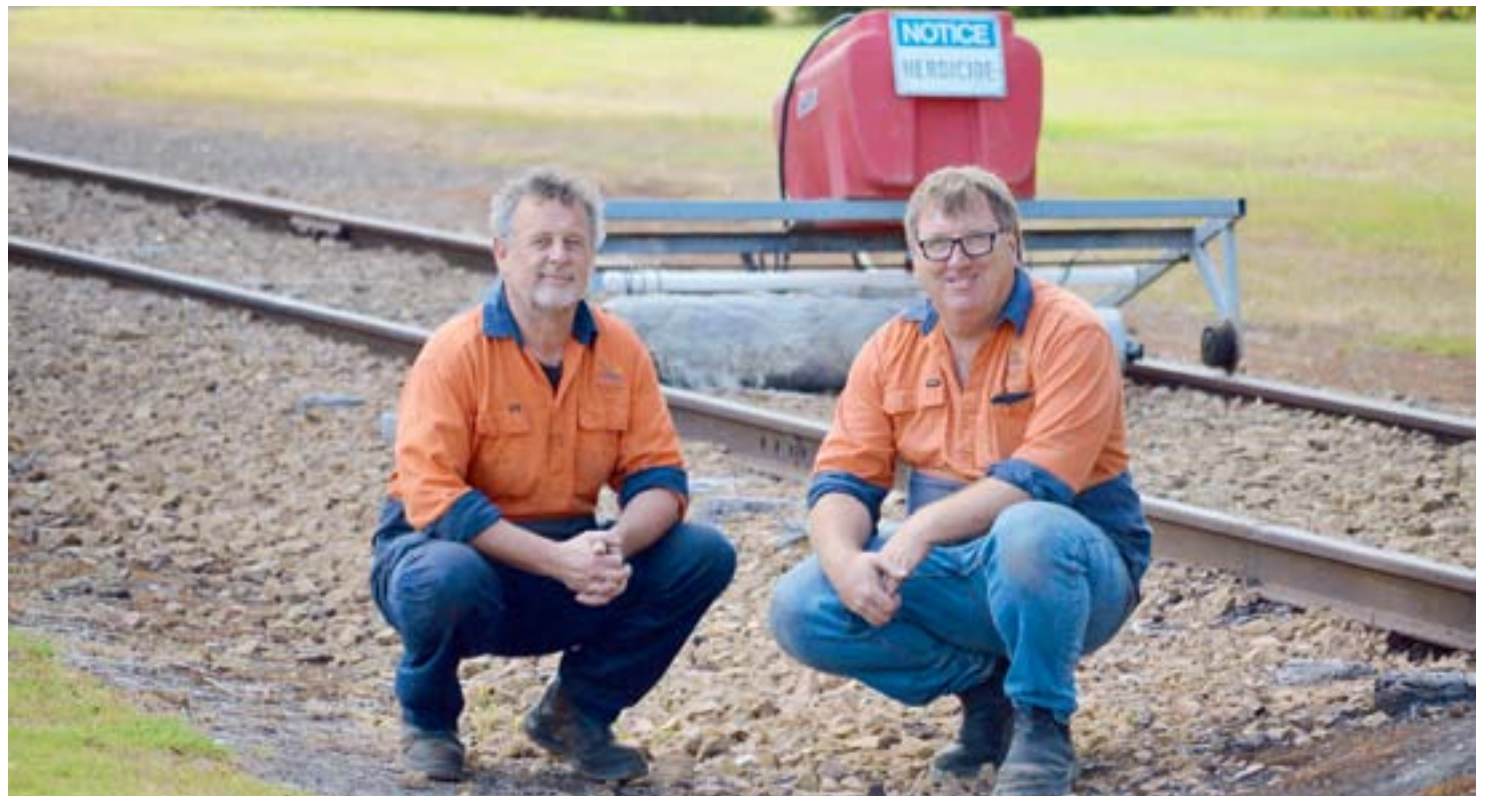
WEED ROLLER: Wattle Range Council mechanics, Andrew Street and Tim Whennen shown with their new invention on railway tracks where it will be ensuring spray drift onto vines does not occur.
