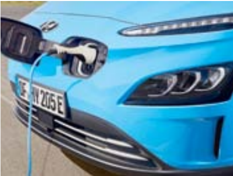
GOING THE DISTANCE: Energy consumption, hence available range, is officially put at a combined 14.7kWh per 100 kilometres, which would allow for 484 km to 'empty'.
